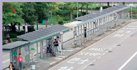
The Kowloon Motor Bus Company (1933) Limited and Long Win Bus Company Limited have installed solar panels on bus shelters to supply electricity for lighting at bus stops
